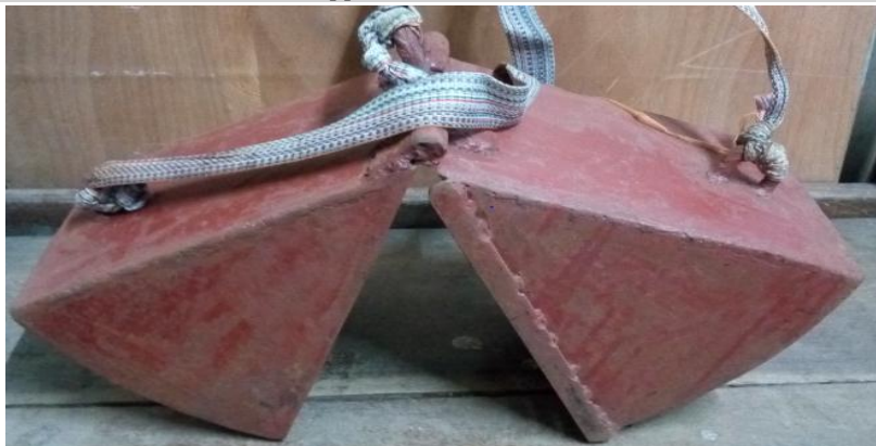
Fig. 2: View of the Ekman type bucket
